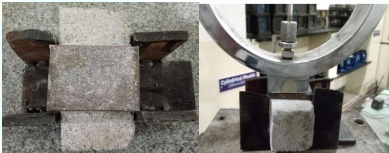
Figure 5. Compressive strength test specimen in zig and test setup
