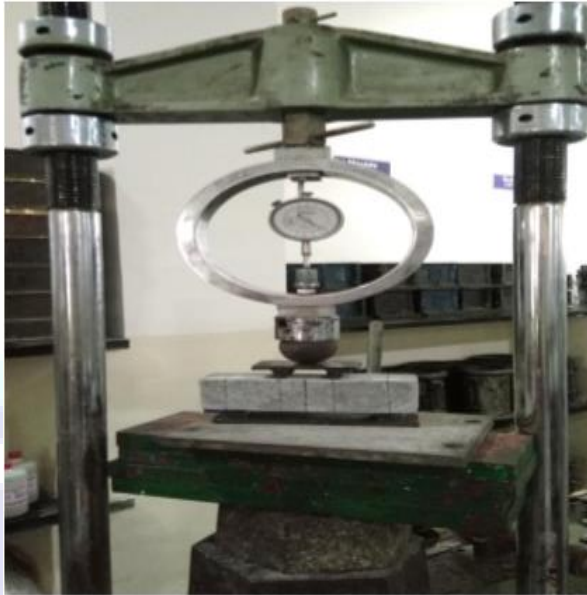
Figure 3. Flexural strength test set up
