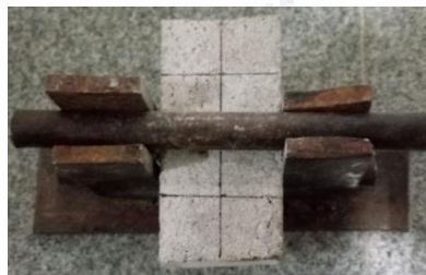
Figure 6. Tensile strength test set up
