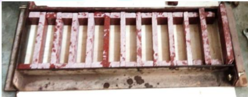
Figure 1. Mould with prism compartments
