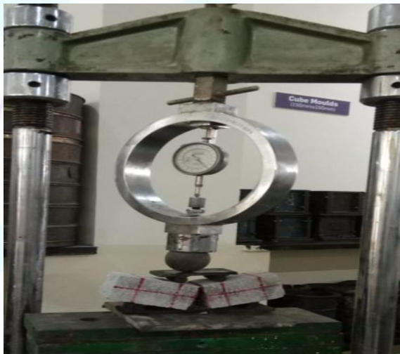
Figure 4. Flexural strength test specimen at failure
