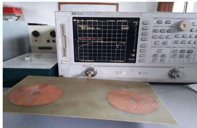
Figure 9: Measurement of Return Loss ( S_{11} ) in network analyzer
