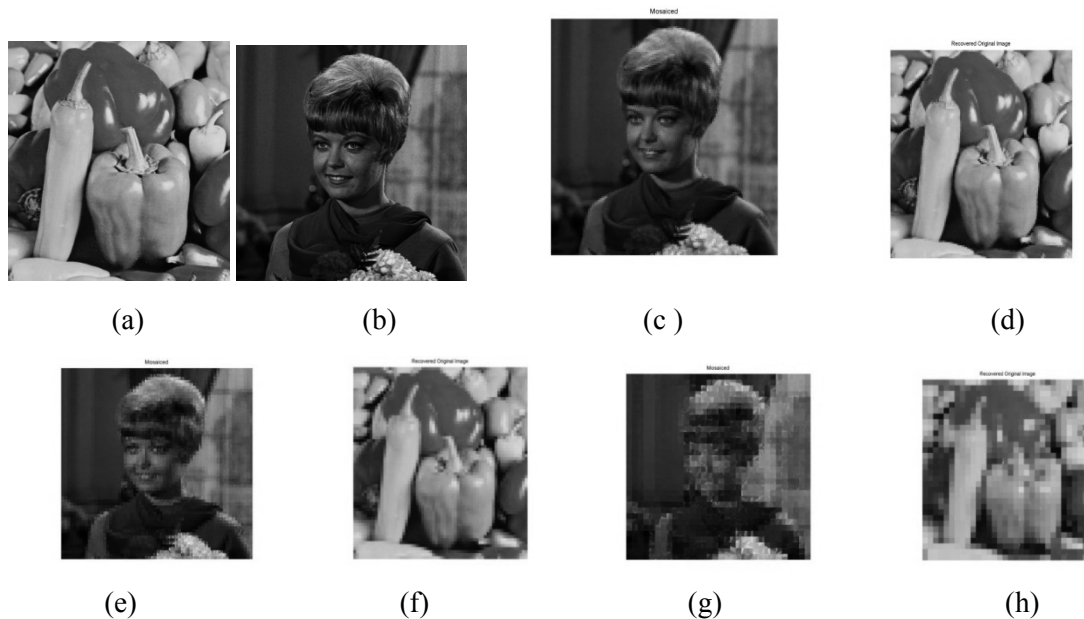
Figure 4.1: Images for Experiment no. 01 (a)secret image (b)target image (c)mosaiced image for block size 4x4 (d)recovered secret image for block size 4x4 (e)mosaiced image for block size 8x8 (f)recovered secret image for block size 8x8 (g)mosaiced image for block size 16x16 (h)recovered secret image for block size 16x16
